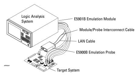
The E5901B emulation module must be used with an E5900B emulation probe.
