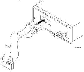
**4** Plug the keyed end of the cable (pin 14 is blocked) into the JTAG debug port on the target system.
