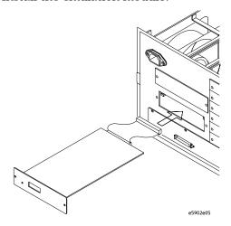
**6** Connect the cable and re-install the screws.
